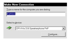
3 Click until you see a window labelled MAKE NEW CONNECTION. Now enter the name you'd like this connection to have, for example, EARTHLINK. The corresponding modem should also be selected; if it's not, select it from the list. Please note: an ISDN device IS a modem! If you're using the Fritz!Card, for example, choose AVM ISDN INTERNET (PPP OVER ISDN). Click NEXT.
